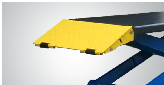
▲ Adjustable ramps and extended platform for longer vehicles.
