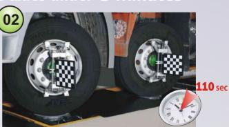
Caster swing can be performed for twin steer axles simultaneously.
