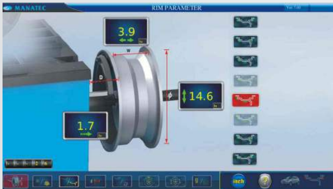
User friendly input screen for entering Rim Parameters.
