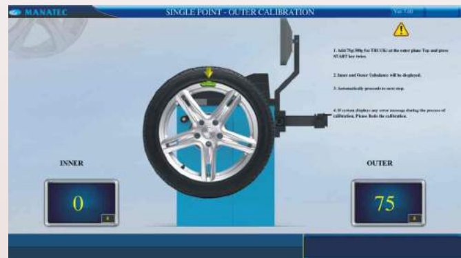
Step by step self calibration procedure guides the user to perform calibration easily & quickly.
