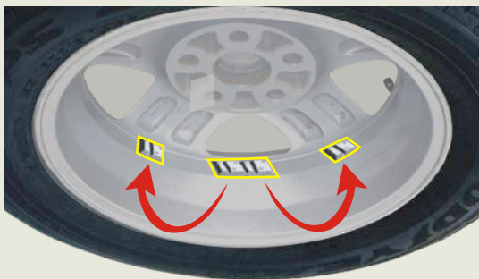
Split weight program (spokes program) helps to split the weight to be hidden behind the spokes of the alloy wheels.
