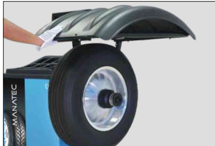
Automatically starts when wheel guard is closed
