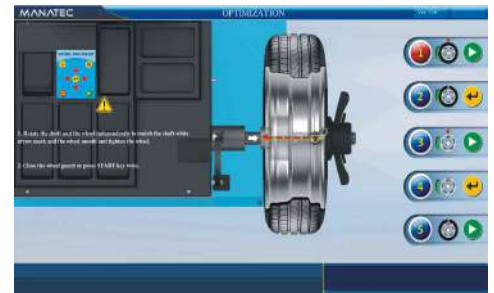
Optimization program helps in reducing wheel weight consumption.
