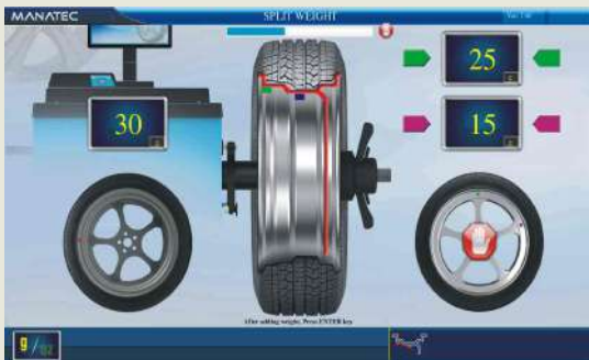
Split weight program (spokes program) helps to split the weight to be hidden behind the spokes of the alloy wheels.
